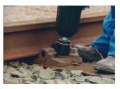
Fitted with a new Roll Bar which reduces vibration; protects the Throttle Handle; provides a foot base for starting and makes the Wrench more comfortable to use.
