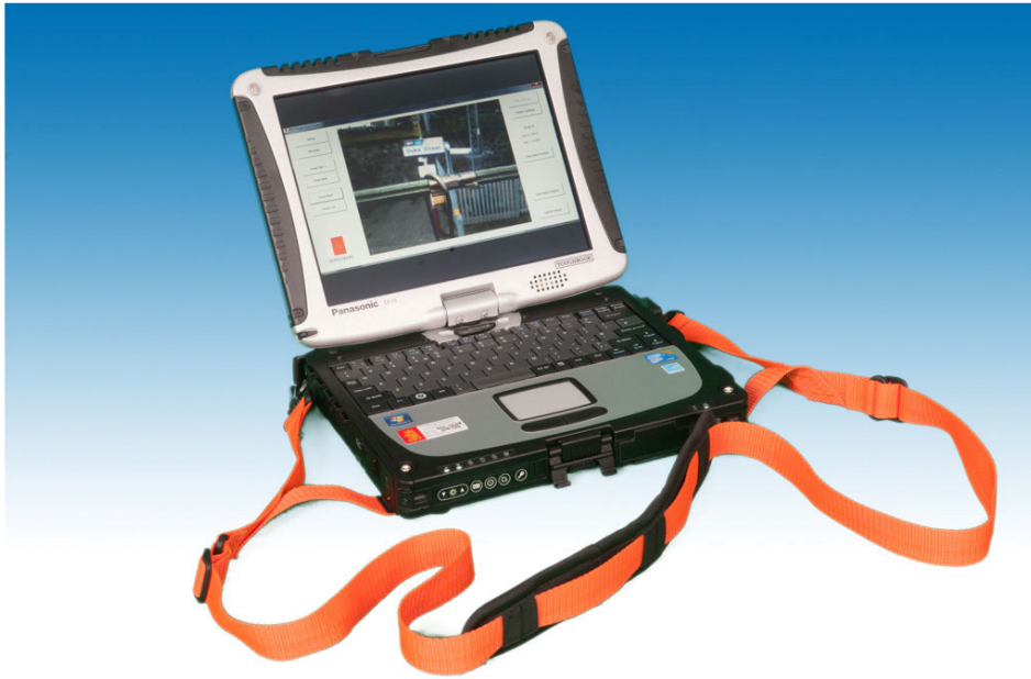
Figure 7- O480-6001 Base Station, Harness and Camera Control Graphical User Interface*
