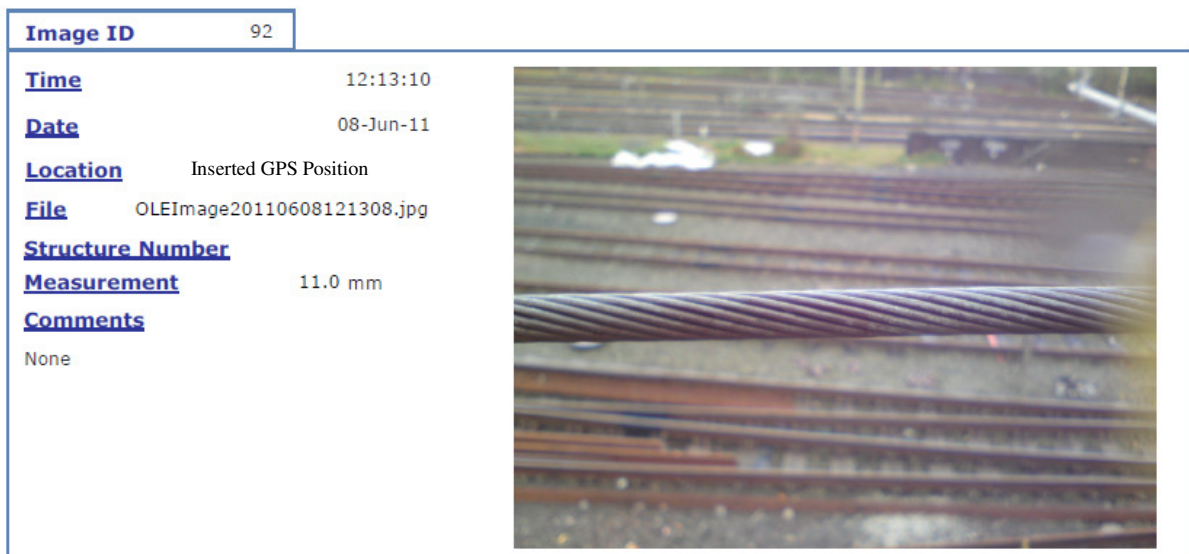
Figure 10 – Example automatic wire survey report template including GPS and wire measurement information. Report templates can be easily customised to suit each client*
