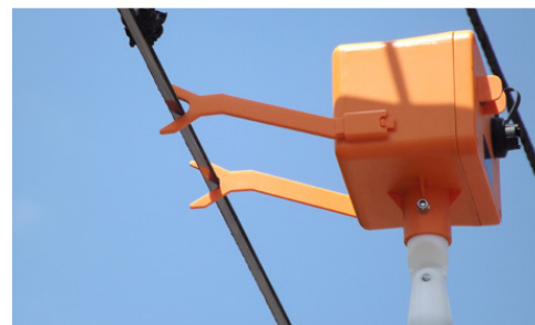
*Figures 1 & 2 - Pole-mounted Inspection Camera, with scaling arms
