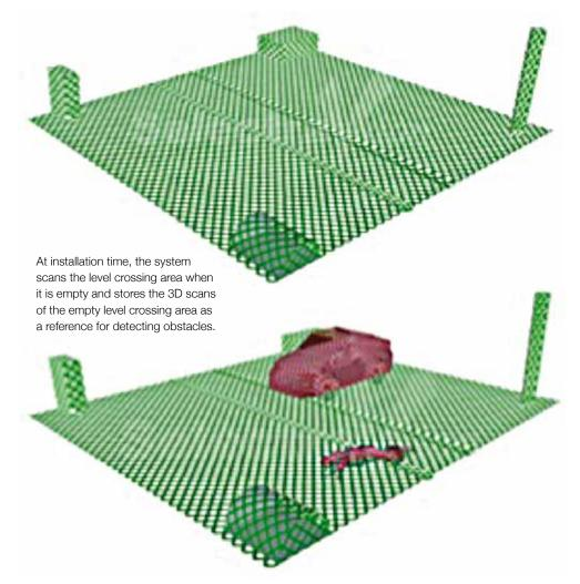
The level crossing obstacle detection system detects all objects in the controlled area of a level crossing, in order to prevent a train colliding with an object such as a vehicle or people on the crossing.
