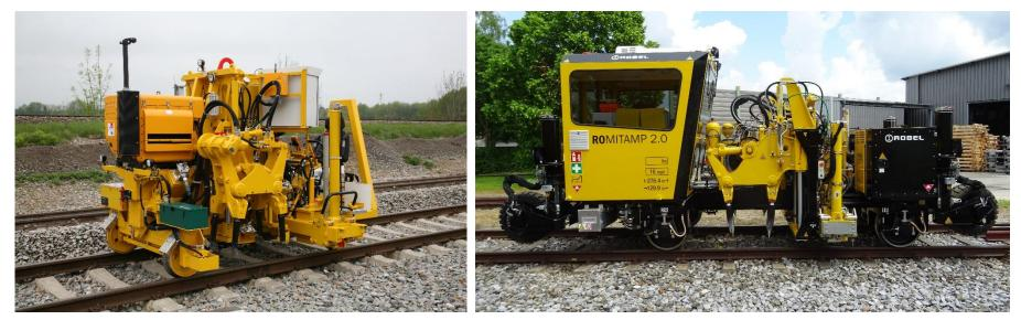
47 kW Engine Weight approx. 5,5 t Speed up to 15 km/h
