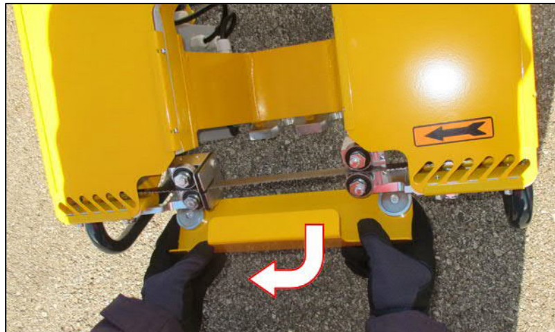
Fig. 31: Removing the transport protection
