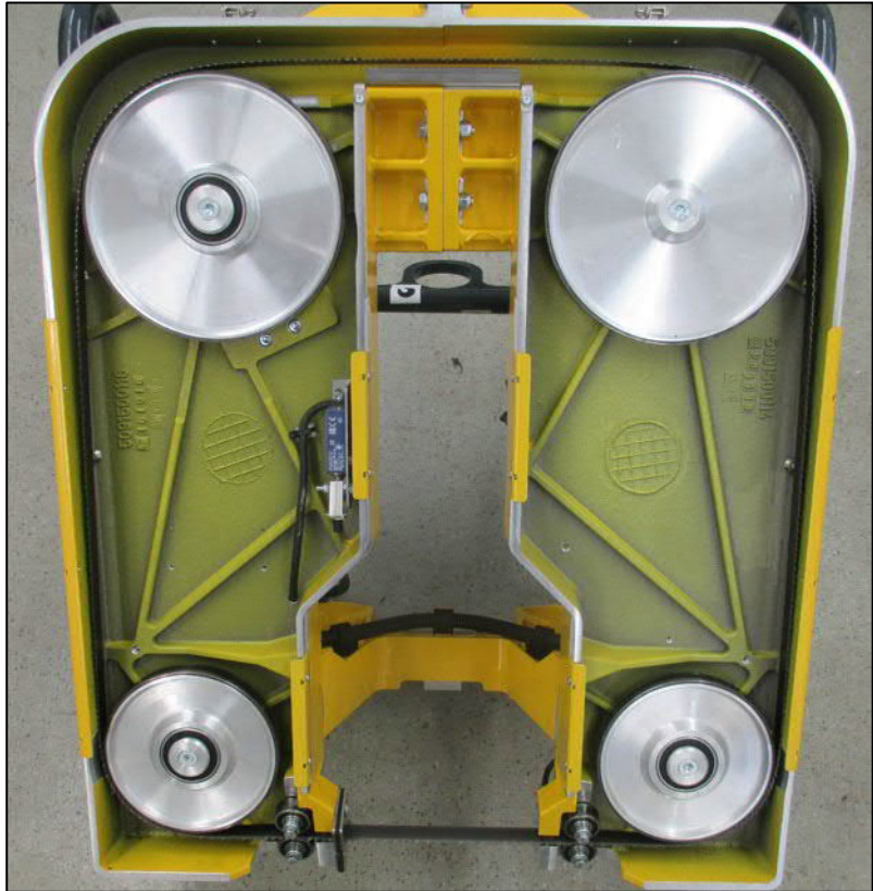
Fig. 39: Inserting the saw band
