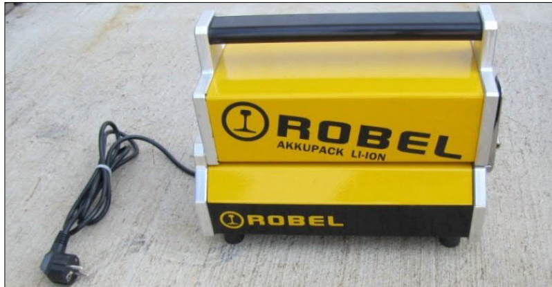
Fig. 8: Charger with attached battery
