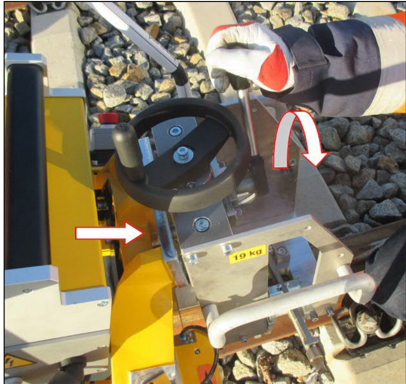
Fig. 34: Mounting the saw unit
