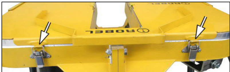
Fig. 40: Closing the quick fasteners
