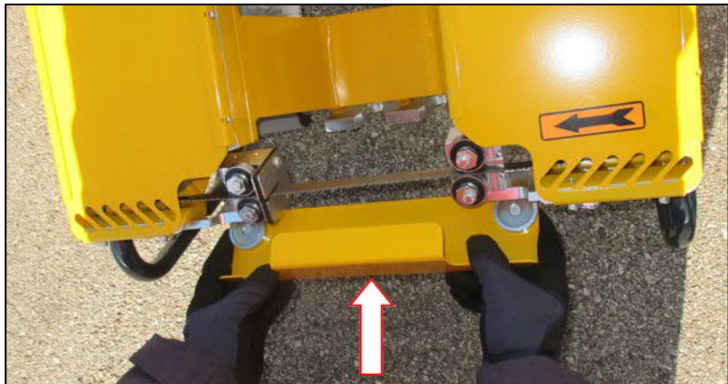
Fig. 42: Fitting the transport protection
