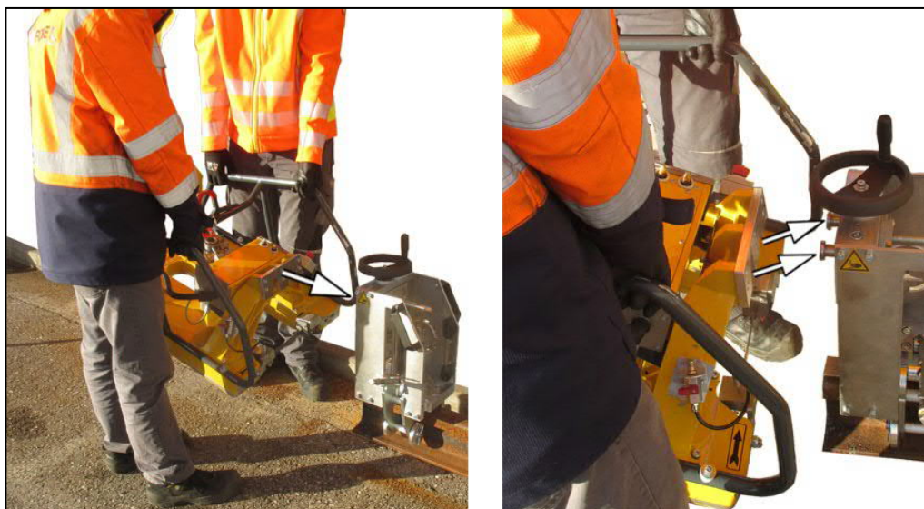
Fig. 33: Fasten the saw unit to the tensioning block
