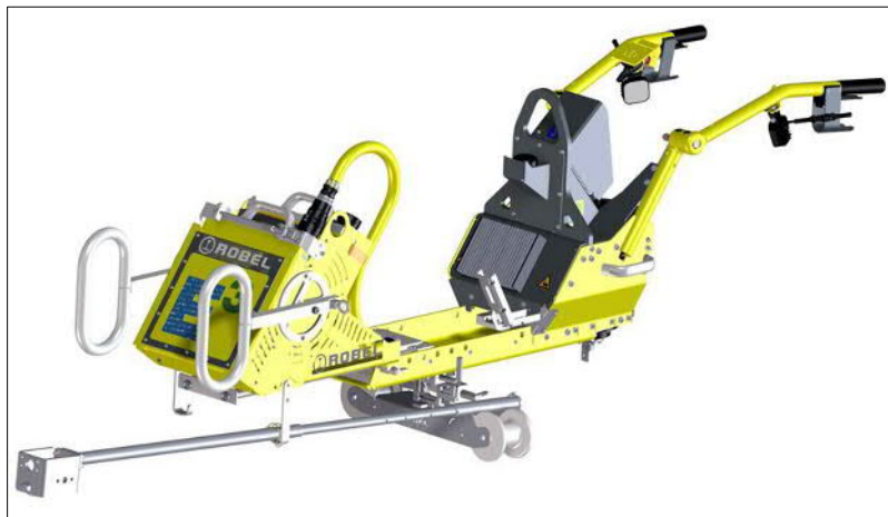
Afb. 115: Cantilever in transportstand
