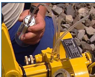
Fig. 74: Fill with oil
