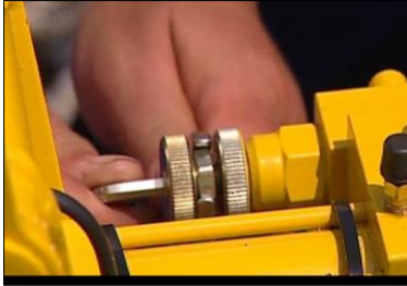
Fig. 78: adjust the knurled screw of the pressure control valve
