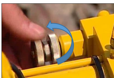
Fig. 73: Open the pressure control valve
