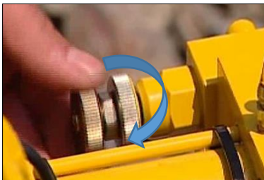
Fig. 77: Close the pressure control valve in stages
